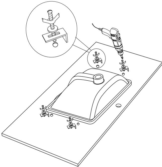
Step 4 Screw the total part on the top and strengthen the part C
